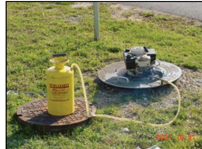
Figure 13. Smoke Testing and Smoke Blower.
