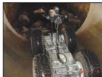
Figure 11. Camera Being Towed (left); Remote Controlled Camera (right).
