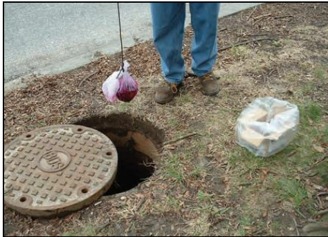
Figure 12. Dye placed into upstream manhole (left); Dye observed at downstream manhole (right).
