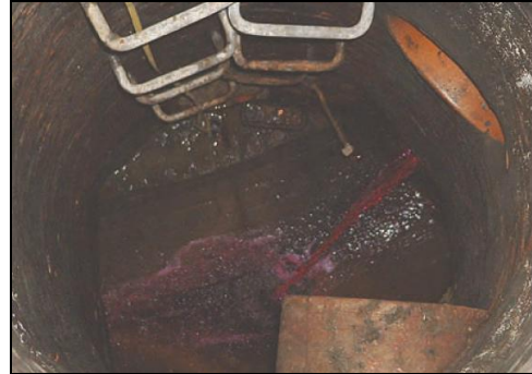
Figure 12. Dye placed into upstream manhole (left); Dye observed at downstream manhole (right).
