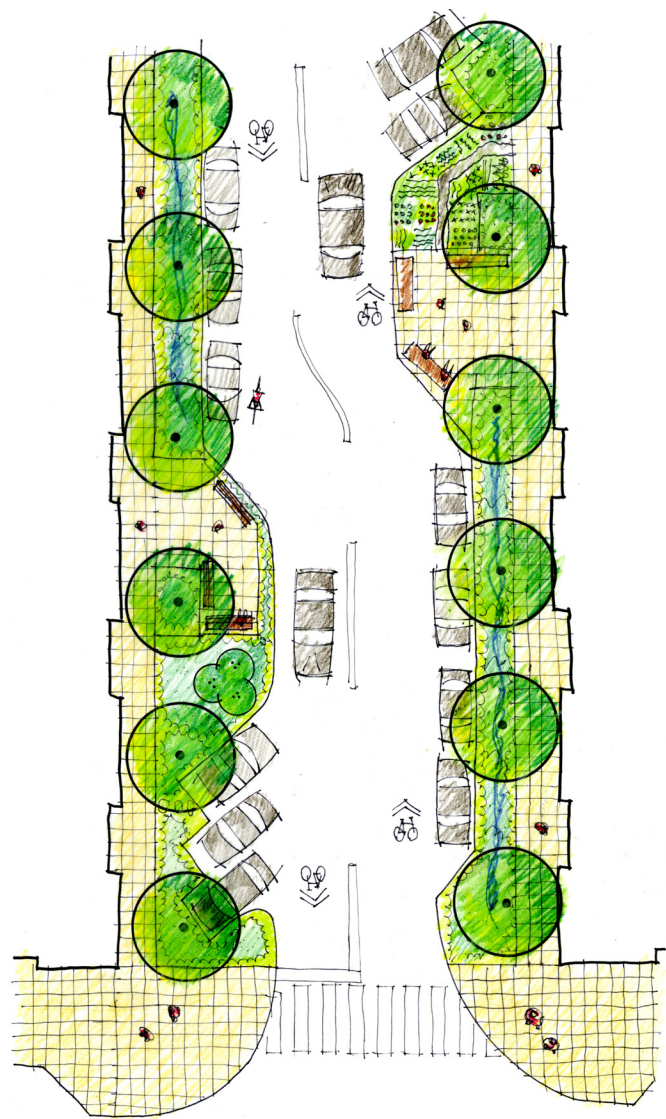
Figure 3.4 Complete Street example with integrated LID techniques including bioretention cells adjacent to “vest pocket” and parallel parking spaces
