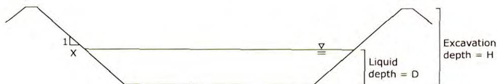
Figure 15. Profile view of typical manure storage lagoon construction. Not drawn to scale; the vertical scale on this diagram is exaggerated to show the side slopes and liquid level clearly.
