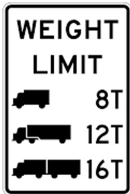
Single Unit – 2, 3, 4, 5, 6, or 7 axles with 8 ton maximum gross weight
