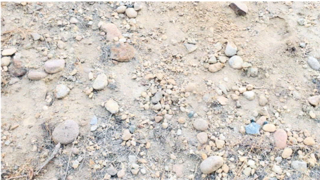
Figure 2: Sandy and gravelly soils observed at the surface of a slope located in the southeastern corner of the discussed parcels. Gravels ranged from approximately 1 to 3 inches in diameter.
