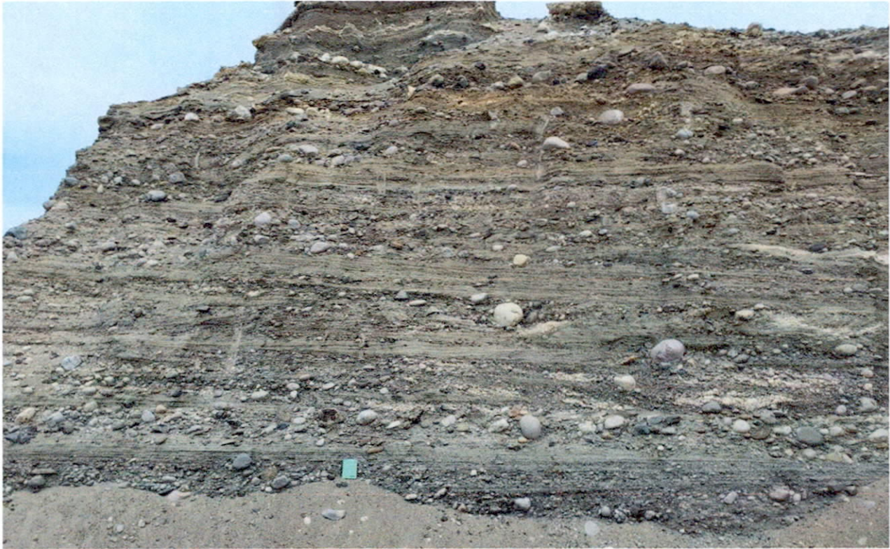
Figure 1: Vertical cut observed near the eastern edge of the current landfill property. Beds of sand and gravel of varying sizes were observed throughout with little silt. Picture facing east.
