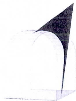
Representative tunnel section illustrating observed wedge
